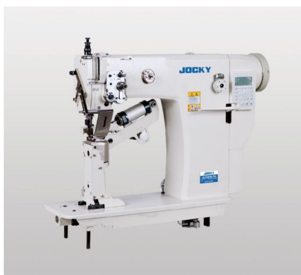
JK1591N-TK 针送料电脑罗拉车(带斩刀) Needle feeding computerized post bed sewing machine (single needle, with tape cutter)
