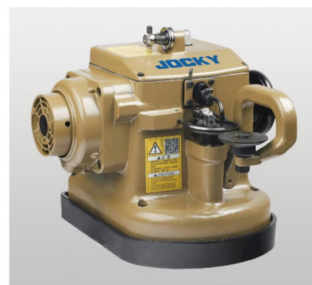
JK2610-5DD 直驱中薄料裘皮机 Direct drive fur sewing machine (for heavy material)
