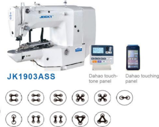
JK1903A-998S 自动送扣钉扣机 (视觉识别系统) Automatic button attaching machine with auto button feeding device (automatic recognition system)
