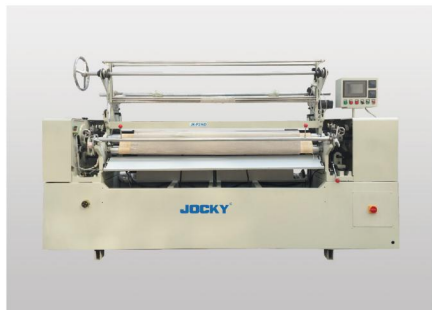
JK-F216D 电脑打折机 Computerized fabric pleating machine
