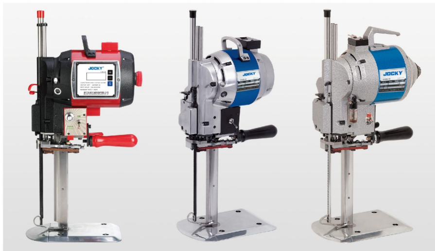
CZD-3E 电脑伺服裁剪机 Computerized servo cutting machine
