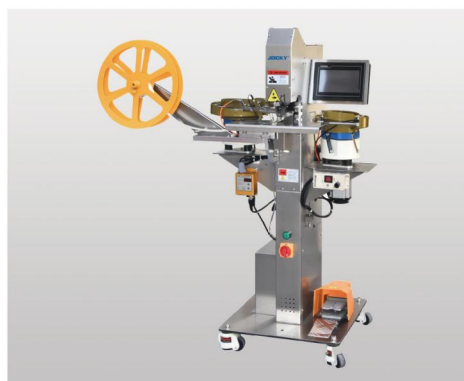
JK-DS90-SKG 全自动打扣机 (西裤扣) Automatic snap button machine (for trousers hook)
