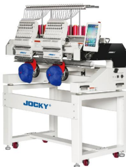
JK-BC1502 双头帽绣机 Double head cap embroidery machine 450x400mm
