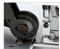
Gear metal roller
