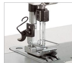
JK390DD-3N 3-needles in triangle
