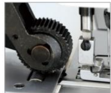
Gear metal roller
